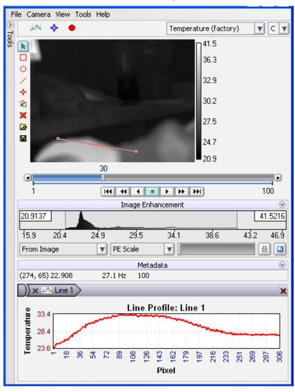
**NOTE:** Plots can be docked to the right and bottom of the initial ResearchIR layout. When a plot is docked, it creates a plot container. New plots can be docked to the top, left, bottom, right, and inside plot containers. In addition, there are two options for docking a plot inside a plot container. As shown in the figure below, selecting the left-
