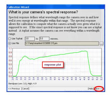
An actual response file should be a **peak-normalized power spectral response** (not a photon response). A response file can be a simple tab-delimitted ASCII file with the wavelength in microns and normalized response values. Below is an example.
