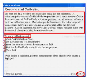
**STEP 9: Add calibration point.** This dialog is used to collect and plot the calibration data. The settings chosen here only affect this calibration point.
