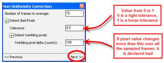
**STEP 3: Collect NUC data.** User will be prompted to fill the field of view with a uniform scene. One or two scenes (hot and cold) will be needed depending on the type of correction being performed. Once you have filled the field of view of the camera with a uniform scene, click "Next". It does not matter which scene (hot or cold) is used first.
