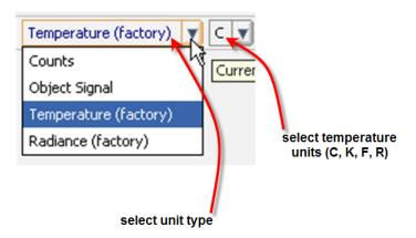
Factory calibrated cameras typically allow:
