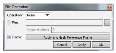
You can use the Extract feature (Sec. 5.9.1.2) to pull a frame from a movie and use as the reference or you can use the Snapshot record function (Sec. 5.7.3) to grab a single frame.
