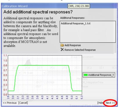
The file format for an additional response file is a simple tab-delimited ASCII file. The first column should be the wavelength in microns and the second column should be the transmission (value from 0 to 1). The data increment does not have to be the same as the spectral response or atmospheric files. ResearchIR will automatically interpolate the values.
