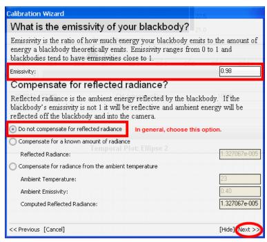
The user can also set options to try and compensate for reflected energy in the scene that is not coming from the calibration source. Typically, this extra source is reflected solar energy. In almost all cases, you should not attempt to compensate for reflected radiance unless you have no other option. If at all possible you should arrange your calibration setup to provide clean, uncorrupted view of the calibration target. This will give you the best and most repeatable calibration.
