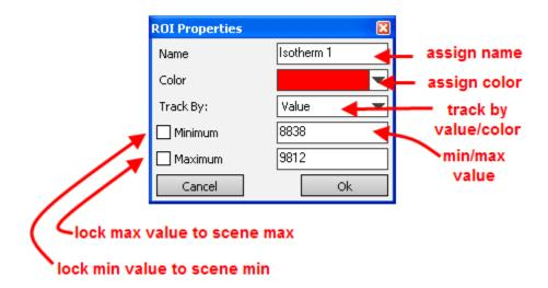
Above isotherms have the max box checked. Below isotherms have the min box checked. Interval isotherms have neither box checked.
