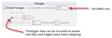
The user can set the buffer size (a tool tip will show the max value for a given computer). The rate limiter options allow the user to slow down the rate of data recorded prior to the trigger. This is useful for extending the time span of the pre-trigger buffer.
