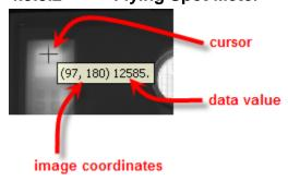
The Flying Spot Meter is a real-time data cursor that appears as the user runs the mouse cursor over the image. To the lower right of the cross-hairs is a tooltip that displays the cursor coordinate (in pixels) and the data value in the currently selected units.
