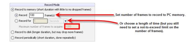
When specifying time it is still necessary to specify a max frame limit. The frame limit can be much higher than the number of frames needed to record the specified time.
