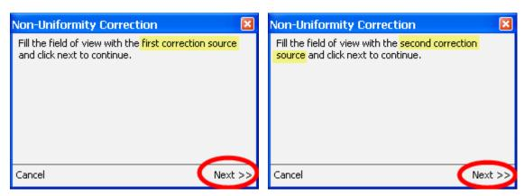
For the best results, the two scenes should be far enough apart in temperature to span as much of the A/D range as possible. If the real scene spans a large range of the A/D than the scenes used to generate the NUC then the NUC algorithm with attempt to extrapolate. This will generally lead to undesirable artifacts in the image.
