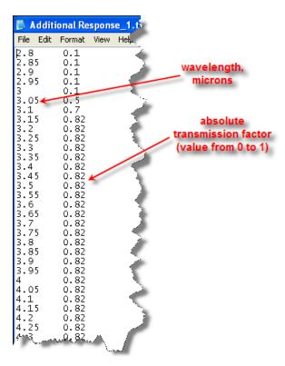
The Additional Response dialog can also be used to input a simple atmospheric path transmission if MODTRAN is not used. In this case only total transmission would be accounted for.
