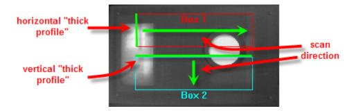
If you open the plot tools by clicking the "<<" icon in the upper right corner of the plot, you can choose the direction and statistic for the thick profile.
