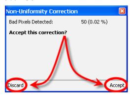
**STEP 5: Enable the PC-Side NUC.** Once you have accepted the NUC, you can apply it to the live image by using the NUC controls next to the Units Selector.
