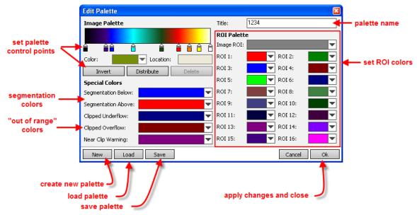
Control Points tell ResearchIR where to start and stop gradients. You can set the color and location of as many control points as you like. ResearchIR will make a gradient between those points. Control points do not have to be evenly spaced.
